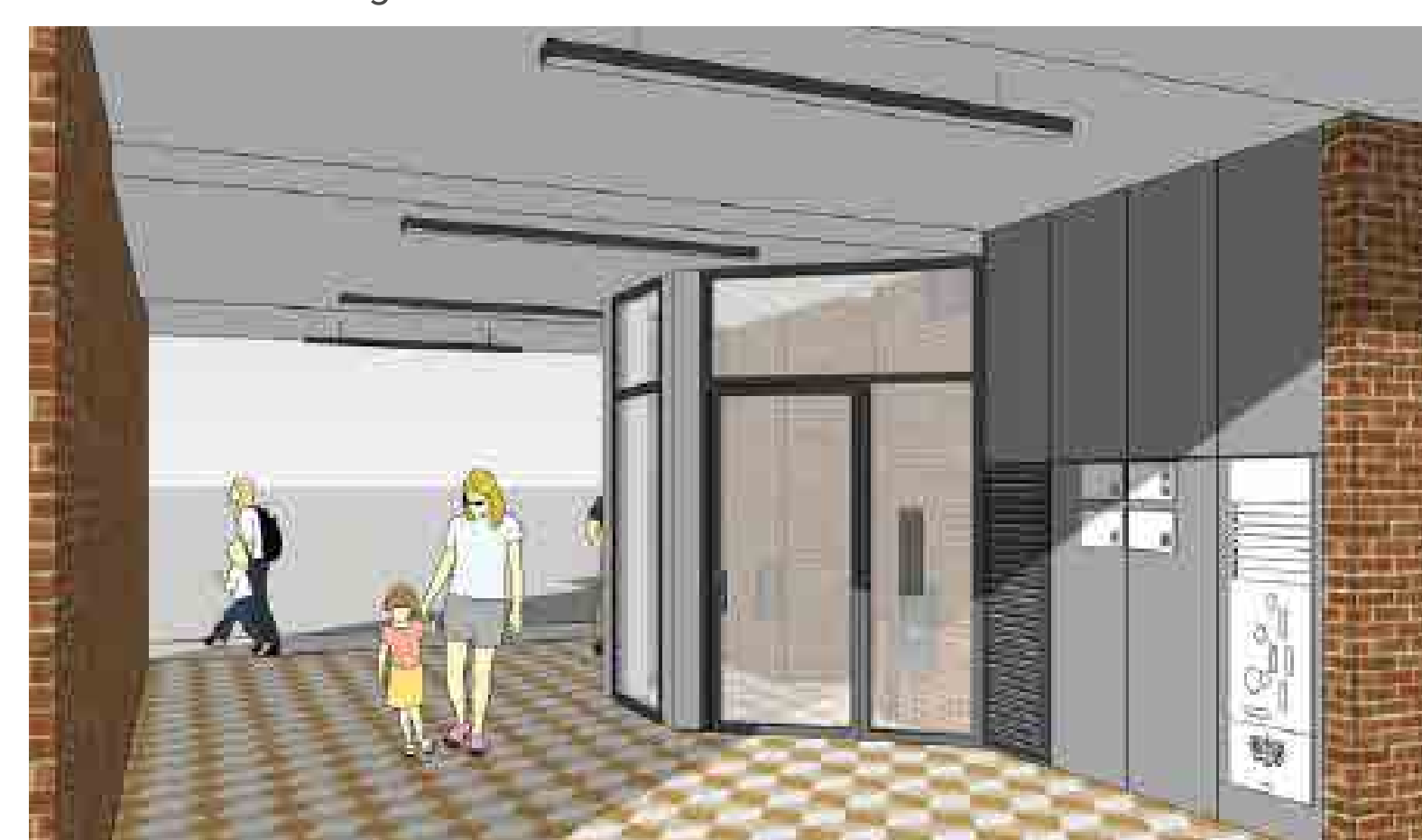
Above: Projecting glazed entrance with parcel boxes and infill panels
